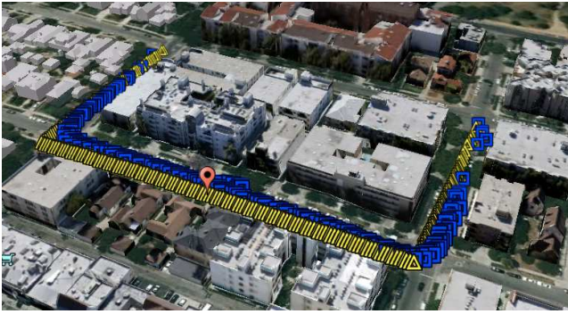
Figure 8: Fixed-to-Mobile experiment: comparison between field experiment (blue squares) and simulation (yellow triangles). Representation of the locations in which the moving car received a packet generate from a source placed in the middle of the road block.
