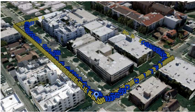
Figure 9: Fixed-to-Mobile experiment: comparison between field experiment (blue squares) and simulation (yellow triangles). Representation of the locations in which the moving car received a packet generate from a source placed at the intersection.
